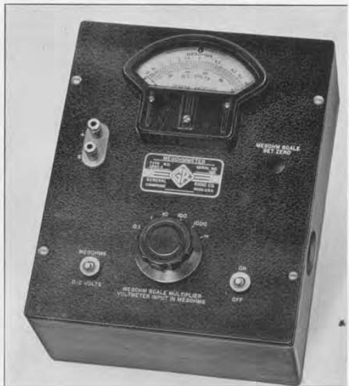
FIGURE 1. Panel view of the TYPE 1861-A Megohmmeter. Superseding the TYPE 487-A, this new instrument measures resistances from 2000 ohms to 50,000 megohms and can also be used as a d-c voltmeter.
